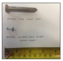
Survey monitoring 'pins' for subsidence monitoring
