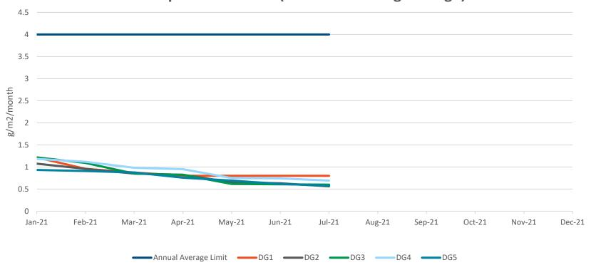
All depositional dust gauges for MC are located around the sites perimeter, no exceedances of long term criteria have been observed year to date.
