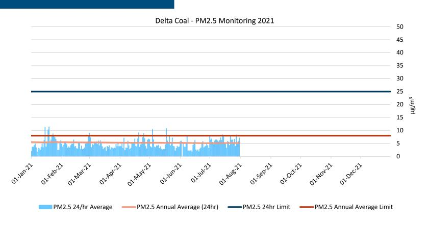
Delta Coal utilises Delta Electricity's Beta Attenuation Monitoring (BAM) PM2.5 continuous monitor.
