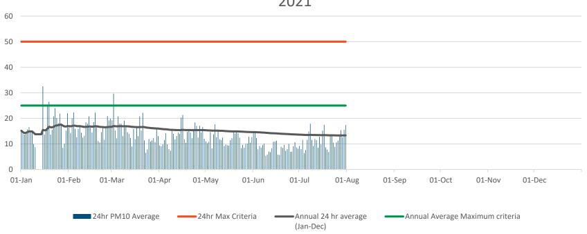
Delta Coals tapered element oscillating microbalance (TEOM) PM10 monitor is located at the Mannering Park Sewage Treatment Plan. No exceedances of the average annual or 24hr criteria have been observed year to date.
